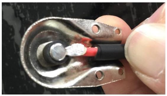
Screw the front shell on ,be careful that the black outer jacket not turn.Please screw tightly. Do the other end then test with cable test or meter then it can work for your pedals.
