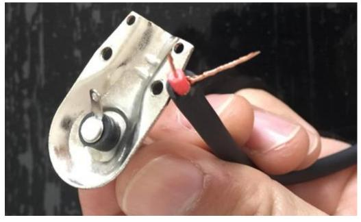
connection like below, the main wire go inside the hole and twist it and the shield should turn back and hide under
