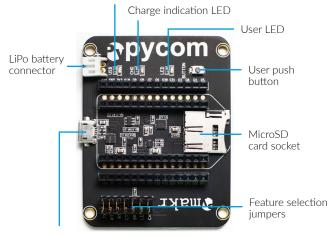
Micro USB connector for power and serieal communication
