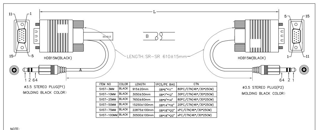
1.CABLE; (A)28AWG(7/0.12TC),NON-UI,NON-FOIL,2C+S,OD=3.0±0.2mm,BLACK COLOR,PVC JACKET. (B)28AWG(7/0.12TC),UL2919,AL+D+B,{[(28AWG\*1C+D+AL)\*3COAX+28AWG\*5.5PAIR]},OD=9.0±0.2mm.BLACK WITH EMBOSS,PVC JACKET.
