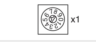
• On the lower rotary switch x1, set the ones digit for the address ("6" in the example).
