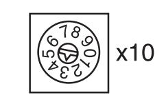
On the upper rotary switch x10, use a small screwdriver to set the tens digit for the address ("3" in the example).
