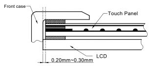
10.2.5 The view area of the touch panel should be at least as large as the view area of LCD, and the active area of the touch panel should be at least as large as the active area of LCD.
