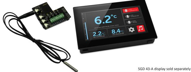
The S43-TP is an accessory to the PanelPilotACE range of compatible displays and panel meters and is compatible with the 4.3" PanelPilotACE display module (SGD 43-A). The S43-TP mounts on the rear of the SGD 43-A and provides up to four thermistor inputs which can then be utilised within the free PanelPilotACE Design Studio software to measure, display, log and graph temperature readings.
