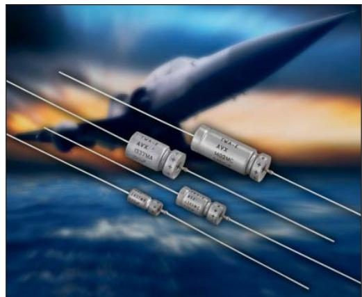
The TWA series is an axial leaded wet electrolytic tantalum capacitor with a unique cathode system that promotes very high CV (Capacitance/Voltage) per cc in traditional MIL-PRF-39006 case sizes.
