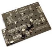
Motor driver and Power distribution board
