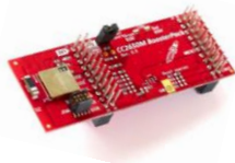
SimpleLink Bluetooth® low energy CC2650 module BoosterPack™ plug-in module
