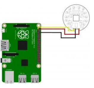
Connect the 5v on the LISIPAROI to the 5v (pin 2) on the Raspberry Pi
