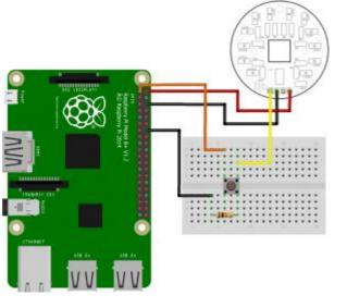
When pressing the button with the Raspberry Pi powered up will turn on the LISIPAROI.
