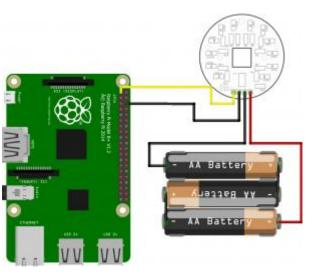
When using an external power supply, both GND (grounds) will be needed, so double check their placements before adding any power to save the risk of damaging the Raspberry Pi or shorting the batteries.
