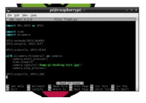
To run the program, type in **sudo python flash.py** followed by enter. The LISIPAROI should switch on, a picture is taken.
