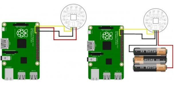
Switch on the Raspberry Pi, and add the batteries (if external power is being used).
