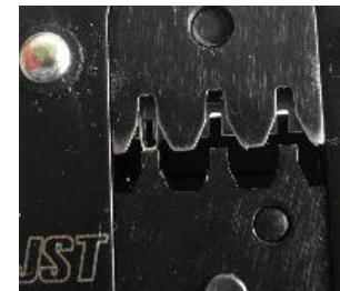
Close the tool lightly until the contact is held (1. Ratchet Lever)
