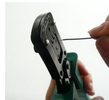
Insert the cable until insulation Stop blade.
