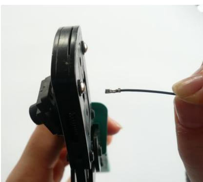
Remove the crimped contact.
