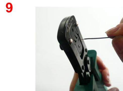
Insert the cable until insulation Stop blade.
