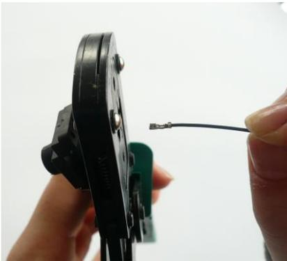
Remove the crimped contact.
