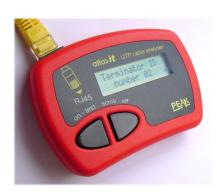
Simply use any number of the *ID Terminators* on one end of each of your network cables (or network sockets by using patch cables). The *Atlas IT* will automatically detect the presence of the *ID Terminator* and display it's identity following the display of the detected cable type (straight through or crossover).
