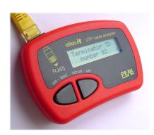
Simply use any number of the *ID Terminators* on one end of each of your network cables (or network sockets by using patch cables). The *Atlas IT* will automatically detect the presence of the *ID Terminator* and display it's identity following the display of the detected cable type (straight through or crossover).
