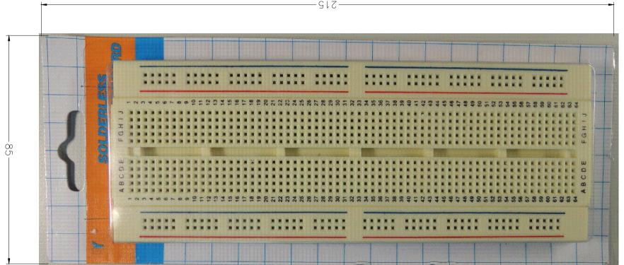
Pitch 2.54mm 2 Distribution Strips, Tie-point 200 1 Terminal Strip, Tie-point 640 Board: 17.3\*6.4\*0.85cm :3TON
