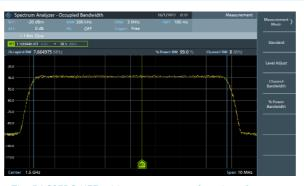
The R&S<sup>®</sup>FPC-K55 adds measurement functions for channel power, occupied bandwidth, spectrogram display, harmonic distortion, TDMA power and third order intercept.
