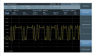
R&S<sup>®</sup>FPC-K7 modulation analysis, including dedicated modes for analysis of Bluetooth<sup>®</sup> Low Energy (BLE) and tire pressure monitoring systems (TPMS).
