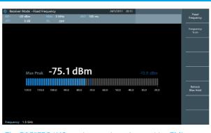
The R&S<sup>®</sup>FPC-K43 receiver mode option enables EMI debugging and includes a quasi-peak detector. Near-field probe sets are available.
