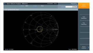
R&S<sup>®</sup>FPC-K42 vector network analysis enables the internal bridge for S11 reflection measurements, including Smith chart and distance-to-fault (DTF).
