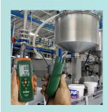
Measures Formaldehyde concentration, Air Temperature, and Humidity. Adjustable audible alarm feature is excellent for checking indoor air quality in buildings.
