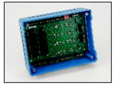
**STA-MB:** The STA-MB Screw Terminal Accessory provides sockets for 4 MB-Series modules. Two parallel 37-pin D male connectors provide interfaces for DAS boards and accessories. The MB-Series module inputs and outputs as well as the I/O connector pins are brought out to screw terminals. You then wire the MB-Series outputs to pins on the I/O connectors according to the requirements of your application.
