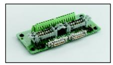
**STA-3108-1 A3:** Adapter panel that adapts the 36-pin connector (from the KPCI-3107/3108 analog I/O port) of the CAB-1284CC cable to four 24-pin headers mounted on the STA-3108A3. Each of these headers has jumpers that are used to select one of four KPCI-3107/3108 input channels.
