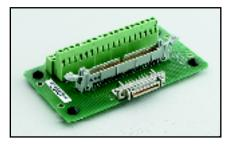
**STA-3108-1 D1:** Adapter panel that adapts the 36-pin connector (from the KPCI-3107/3108 digital I/O port) of the CAB-1284CC cable to a 50-pin header (mounted on the STA-3108D1) with signals arranged for use with KPCI-PIO96 accessories.
