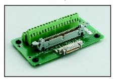
**STA-3108 A1:** Adapter panel that adapts the 36-pin connector (from the KPCI-3107/3108 analog I/O port) using the CAB-1284CC cable to a 50-pin header mounted on the STA-3108A1.
