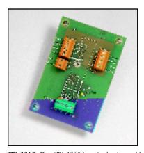
**STA-1360:** The STA-1360 is a single-channel backplane for the MB-Series modules. It accepts one MB-Series module. All connections are brought out to screw terminals. It can be used in applications where only one signal conditioning module is needed or as a convenient adapter for test or evaluation purposes. Standoffs are included so the board can be easily located on any flat surface. Includes 34 " standoffs.
