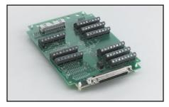
**STA-300:** Screw Terminal Accessory. Mounts on a panel and includes nylon standoffs for tabletop applications. Requires a CAB-305 cable.
