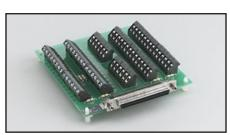
**STP-68**: Screw Terminal Panel. The STP-68 brings all signals out to external screw terminals. Requires a CAB-305 cable. Not CE approved.
