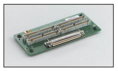
CONN-3160-D1: Screw Terminal Panel. The CONN-3160-D1 Adapter Panel brings all KPCI-3160 digital I/O signals out to an external panel via 50-pin headers. This panel allows connection of the ADP-5037 to allow the KPCI-3160 to operate the SRA-01 or ERA-01, ERB-24 or SSIO-24 relay products or to allow digital connections via the STP-50 or STA-50 Screw Terminal Panel and accessory boards. Requires the CAB-1800 or CAB-1800/S cable.
