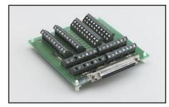
STP-3140: Screw Terminal Panel. Brings all KPCI-3140 signals out to external screw terminals. The STP-3140 comes with nylon standoffs, making it ideal for placing on a desktop or mounting in custom panels. Requires CAB-305 cable (1m/39").
