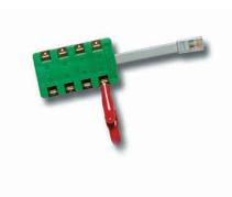
The MA2/RJ45 alligator clip/hook contact is now becoming the standard for ISDN and is now becoming the standard for all structured cabling systems and networks. It is supplied as a USA and international 8/8 plug.
