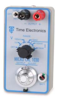
The **1030** is a compact, low cost, portable voltage and current calibrator for general purpose signal injection. It is suitable for voltage and current loop signal simulation as well as thermocouple simulation. The precision 10-turn dial provides a conventional feel to setting the output with a setting resolution of 1 part in a 1000 (0.1%)
