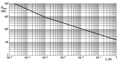
Pulse on a regular basis; maximum permissible peak pulse power  $\hat{P}_{max}$  as a function of pulse duration (t<sub>i</sub>) for single pulse condition
