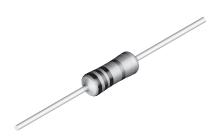
A metal glazed film is deposited on a high grade ceramic body. After that caps are applied to the rods and tinned electrolytic copper wires are welded to these end caps.
