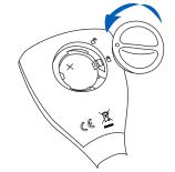
To change the CR2032 Li-ion battery, turn the battery cover located on the back of the meter counterclockwise to unlock. Remove cover and replace with + side facina up.
