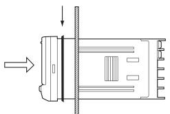
**3.** Fit the adaptor into the grooves on the left and right sides of the rear case, then push it until it contacts the panel to secure the K3MA-L.
