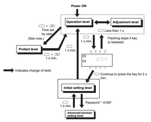
Note: The move-to-protect-level time can be set in the advanced-function setting level.
