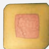
Micrograph of a square crimp
