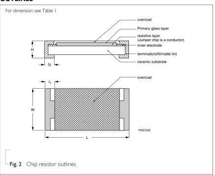
Chip Resistor Surface Mount RC SERIES 0402 (RoHS Compliant)
