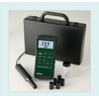
Complete with 0.8" (20mm) probe on 13ft (4m) cable, membranes, protective holster with stand, 9V battery, and carrying case
