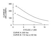
One cycle is 360° rotation and a return through all switch positions to the starting position. The data for the curve was measured at sea level, 25°C and 68% relative humidity with the following limiting criteria:
