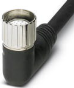
Socket M23, angled, 19-pos., with 15.5 m master cable
