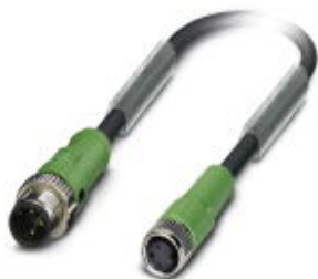
Sensor/actuator cable, 3-position, PUR halogen-free, black-gray RAL 7021, Plug straight M12 SPEEDCON, A-coded, on Socket straight M8, cable length: 0.6 m
