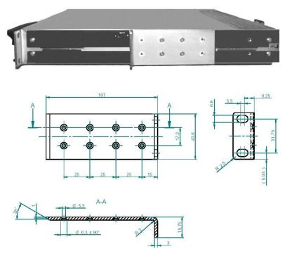
Center Angular Bracket sets can be ordered: Bel Power Solutions part no.: HZZ01222 Note: Each Center Angular Bracket set contains 2 brackets and 8 screws. Filler for covering of the empty shelf slots
