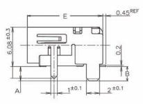
Right Angle Surface Mount Header with Flange (Long Body)
