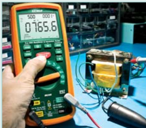
Measure the insulation resistance of transformer windings
