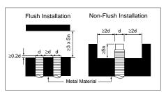
General Mounting – You must maintain minimum distance between adjacent and opposite sensors in addition to non-target metals as specified in the drawings above. Flush mount sensors must extend at least 0.2 times the sensor diameter above the adjacent metal housing. Non-flush mount sensors must extend a distance greater than the sensing distance (Sn). Please contact Altech for any installation assistance
