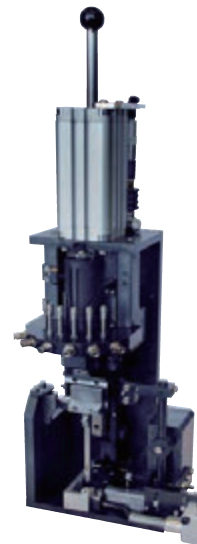
Pneumatic Insertion Tool
