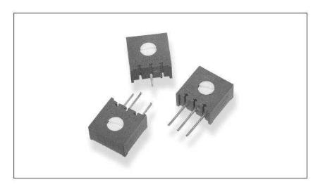
These long established 10mm square, single turn potentiometers will meet wide range of industrial and professional applications. Cermet element technology ensures stability and reliability. This P.C.B. mounted package has easy top or side adjustment, or finger adjust styles. All components are sealed to withstand printed circuit board washing solvents.
