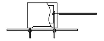
Temperature monitored inside the capacitor.
