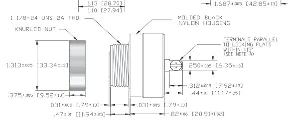
NOTE A: TERMINALS-.032 BRASS TIN PLATED, TAPPED FOR #6-32 SCREW. TWO #6-32 NICKEL PLATED BRASS SCREWS INCLUDED. WILL ACCEPT 1/4" QUICK CONNECT
