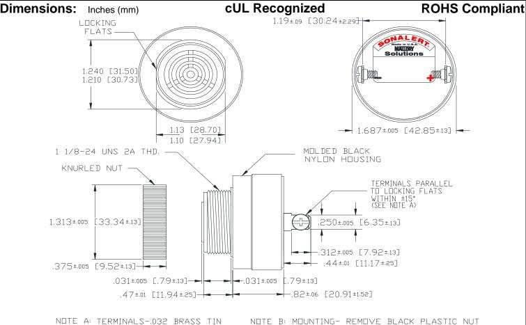
PLATED, TAPPED FOR #6-32 SCREW. TWO #6-32 NICKEL PLATED BRASS SCREWS
