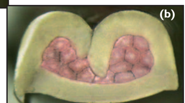
Significant flash can be generated with excessive anvil to crimper clearance, as shown by nominal design condition (a) and +0.003 in over nominal condition (b)
