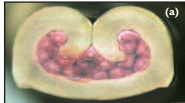
Cross Sections Showing Minimum (a) and Maximum (b) Area Index per Terminal Specification—a Variation of \pm 3.5\%
