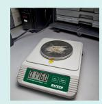
Professional electronic counting and weighing scale with load cell transducer for high accuracy and performance. Wide capacity measuring single small electronic component weighing 0.005oz (0.1g) or batches up to 21.164oz (600g). Optional software available for generating reports and documentation of inventory components.
