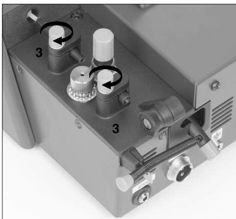
**3.** Place the tubes and guides set in the control unit. Note: with the **0,4 - 0,5 Ø** guide set is necessary to extract the wire of protection. Tighten the screws.
