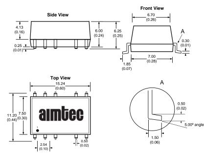
All dimensions are in mm (inch) All Pins are on a 2.54mm (0.10inch) pitch with tolerance of  $\pm 0.25$ mm (0.01inch)
