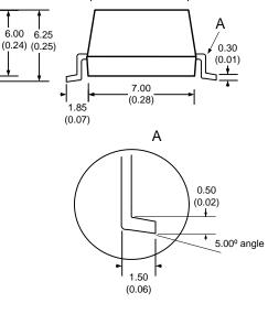
All dimensions are in mm (inch) All Pins are on a 2.54mm (0.10inch) pitch with tolerance of  $\pm 0.25$ mm (0.01inch)
