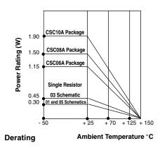
"A" PROFILE + 70 °C PACKAGE RATINGS CSC12A 1.5 W CSC11A 1.37 W CSC10A 1.25 W 1.12 W CSC09A CSC08A 1.00 W CSC07A 0.87 W CSC06A 0.75 W CSC05A 0.62 W CSC04A 0.40 W
