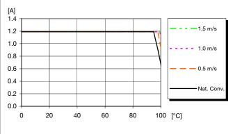
Available load current vs. ambient air temperature and airflow at  $V_{\rm I}$  = 53 V. See Thermal Consideration section.
