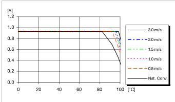
Available load current vs. ambient air temperature and airflow at V<sub>I</sub> = 53 V. See Thermal Consideration section.
