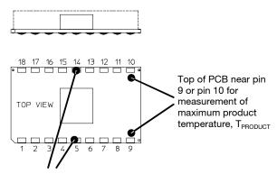
Pin 5 of pin 14 for measurement of minimum pin (solder joint) temperature,  $T_{\text{PIN}}$
