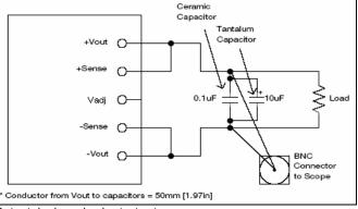
Output ripple and noise test setup
