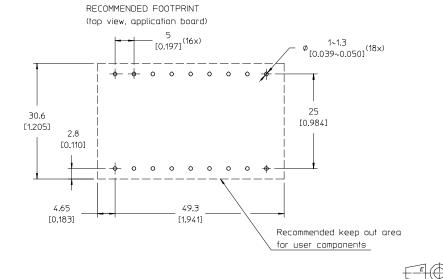
Weight: typical 11 g All dimensions in mm (inch) Tolerances unless specified x.x mm ±0.26 (0.01), x.xx mm ±0.13 (0.005) (not applied on footprint or typical values)
