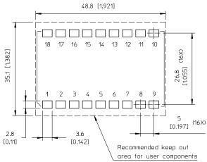
The recommended footprint (see previous page) is optimised for the solder bump design. However, the standard PKF footprint will also accomodate this solder bump design. The only differences is the solder pad width (2.8 versus 2.3 mm) and the c-c distance between the two rows of solder lands (26.8 versus 26.6 mm).
