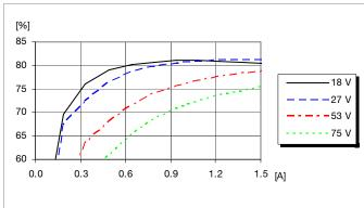
Efficiency vs. load current and input voltage at  $T_{ref}$  = +25°C
