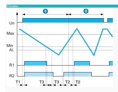
On power-up, probes Min, Max and Al. are submerged, relays R1 and R2 are energised and the pump is ON: emptying starts, the LED for relay R1 is lit. When the Min probe emerges, relay R1 goes off. If, in the event of a fault, the level continues to fall and probe Al. emerges, relay R2 de-energises and the alarm is triggered: the LED relay R2 is lit. This fault can be stored.
