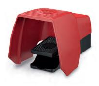
Standard OFF-ON Operation -Push forward in the Anti Trip Pedal Lock to release. Push down pedal to change contact state. Release pedal to return to original state. Standard OFF-ON Operation -Push pedal to change contact state. Release pedal to return to original state. With anti-fatigue footrest. Foot Switches with built in ASI Bus System interface via an M12 plug connection. Available in Standard or Enabling Switch versions
