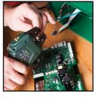
Adjustability: PowerSense<sup>™</sup> technology allows the user to hold and adjust material for ideal positioning before crimping.
