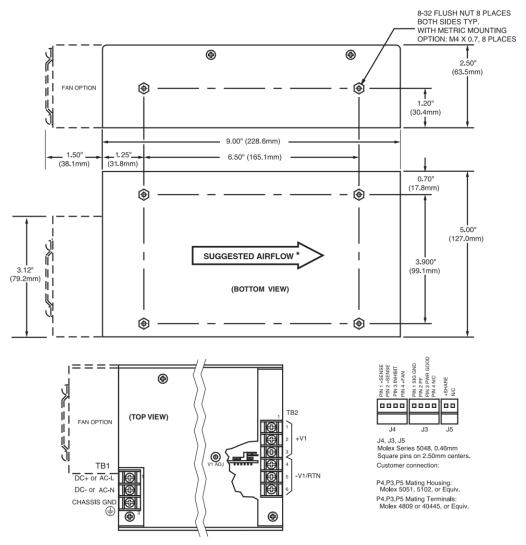
Input and Output Connections: 6-32 Screw Terminal on 0.375" (9.5mm) centers
