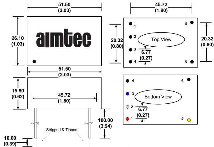
\*Lead Wires are under the specifications of general lamps: \*Wire is UL 1015/CSATEM listed #22AWG / 600V / 105°C
