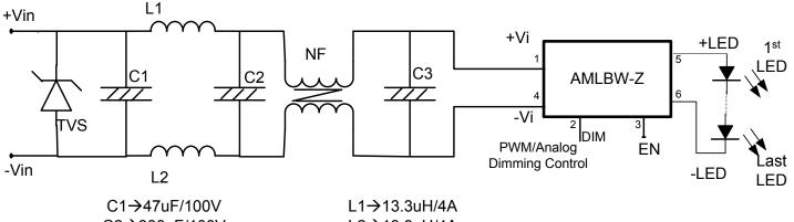
C1→47uF/100V C2→330uF/100V C3→330uF/100V TVS→38V
